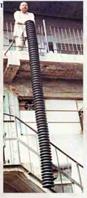
The construction of these bellows includes fabric and elastomer, which is formed from the desired elastomer mainly from NEOPRENE to get better ozone resistance as well as chemical resistance. Also selected polymers can provide required properties. These bellows are stitched indiudually to get better strength and to get maximum life of the same.
